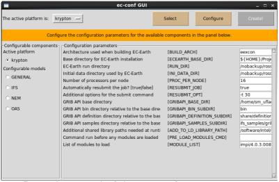
Configuration panel of the ec-conf GUI
